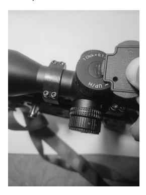
Once the cap is removed turn it over so that the internal components are visible.
