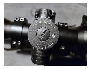
Another feature that I want to point out in this review is the turret rotation indicator, this is an extremely useful tool when shooting at extended ranges where elevation adjustments require more than one full rotation of the elevation turret. Simply passing your hand over the elevation turret, lets you know that you should be looking at the top line numbers of the turret cap.
